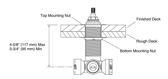
☐ Drill a 1-3/8" (35 mm) hole at the diverter installation location.
