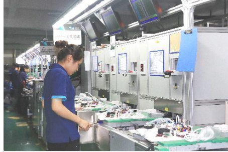
Seat base 100% aging test
