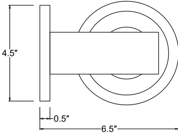
**This fixture can be mounted with shade pointing upward or downward**
