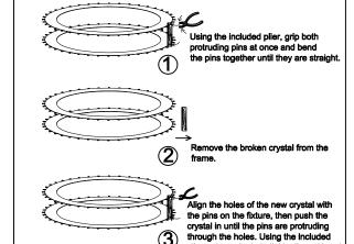
plier, grip each pin individually and bend outward, away from the other pin, until the crystal is secure.
