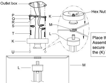
Place the (M) Fabric shade and (K) Top Assembly onto the top of (L) Frame, then secure them by tightening the hex Nut of the (K) Top Assembly.
