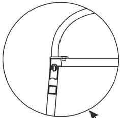
Make sure that the iron tubes are assembled straight relative to the top and bottom ring before tightening the top screws and the bottom finials.
