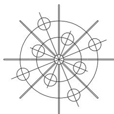
SPREAD THE FIXTURE ARM AND ARM RING TO A SUITABLE POSITION
