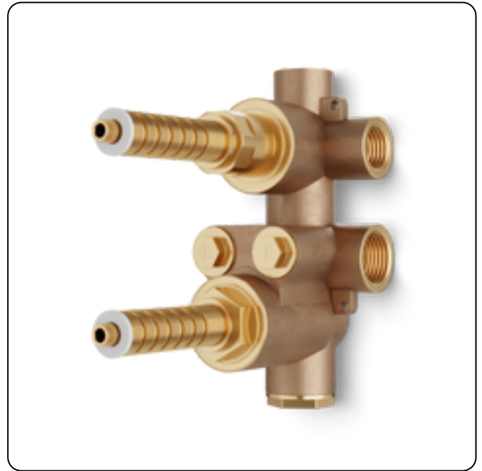
F973ANSVO: 3/4" Thermostat Valve with 3-Way Non-Shared Diverter & Off Position
