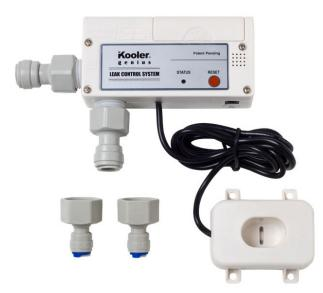
The Safety Valve is a leak detector that, when hooked to a water inlet line, automatically shuts off the water source if it detects moisture. Once the valve shuts off, the unit sounds off with an audible alarm like a smoke detector to let you know of a problem. The unit doubles as a standard shut-off for water filter cartridge replacement and is easy to install. We recommend using a safety valve for any of our filtration faucets for the cleanest and safest installation.
