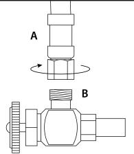
Before connecting supply hoses, flush supply stops to clear any debris. Place a bucket underneath stops and run water for 5 to 10 seconds. Turn water off.
