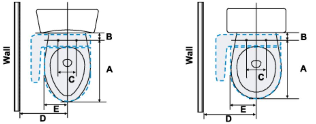
**Note:** Some styles of toilets may not allow the Washlet C110 to be installed due to certain contours near the tank and bowl area (see figures below). In the figure on the left side below, dimension D does not allow for enough open space to accommodate the minimum width of 11 inches.
