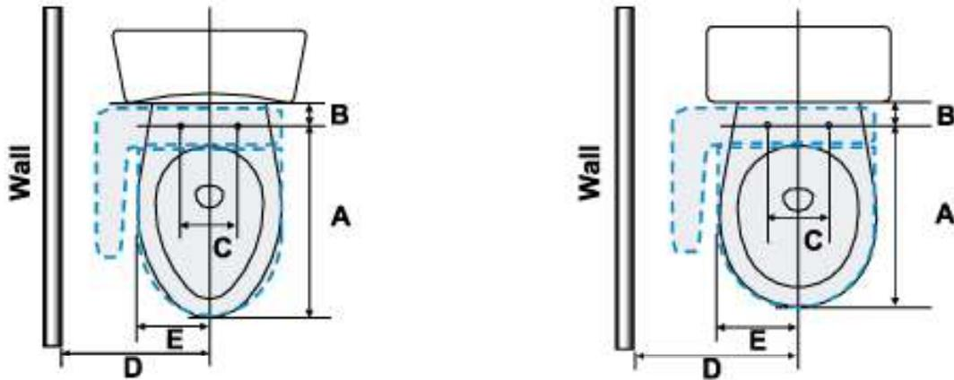
**Note:** Some styles of toilets may not allow the Washlet B100 to be installed due to certain contours near the tank and bowl area (see figures below). In the figure on the left side below, dimension D does not allow for enough open space to accommodate the minimum width of 11 inches.
