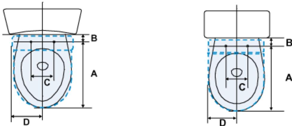
**Note:** Some styles of toilets may not allow the Washlet E200 to be installed due to certain contours near the tank and bowl area (see figures below). In the figure on the left side below, dimension D does not allow for enough open space to accommodate the minimum width of 9 inches.
