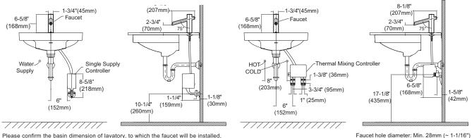
Please confirm the basin dimension of lavatory, to which the faucet will be installed, making sure that it has recommended minimum dimensions of (L x W:  $15" \times 15"$ ).
