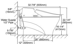
Drain pipe installation position
