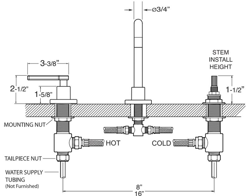
NOTE: Spout and valves install through 1-1/4" diameter holes
