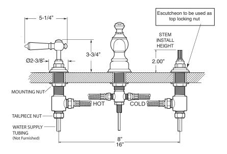
**NOTE:** Spout and valves install through 1-1/4" diameter holes
