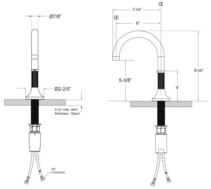
**NOTE**: Spouts install through 1-1/4" Diameter Holes.
