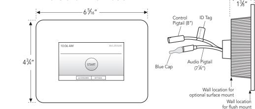
iSteam controls flush mount in the steam/shower enclosure through a 5-1/4" wide x 3-9/16" high hole. iSteam controls can also be surface mounted. They are suitable for use with an available iGenie® control. Available in black or white.
