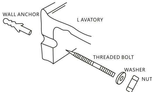
\* For wood stud installation, same as above but without the wall anchor.
