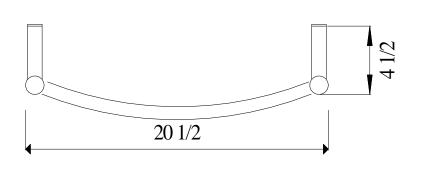
For construction with wall studs on 16 in. centers, the header is located between the studs for the right side mounting. For construction with wall studs on centers greater than 19-1/2 in. provide secure header as shown.
